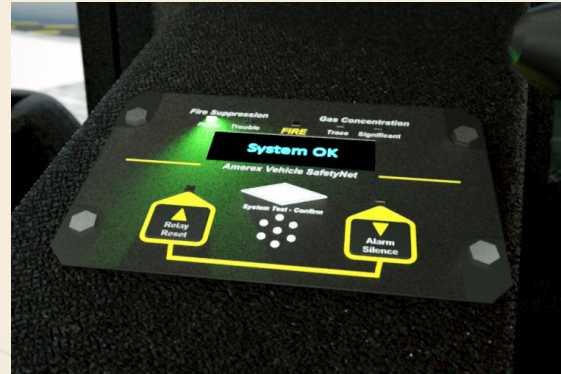
SafetyNet Display Panel
